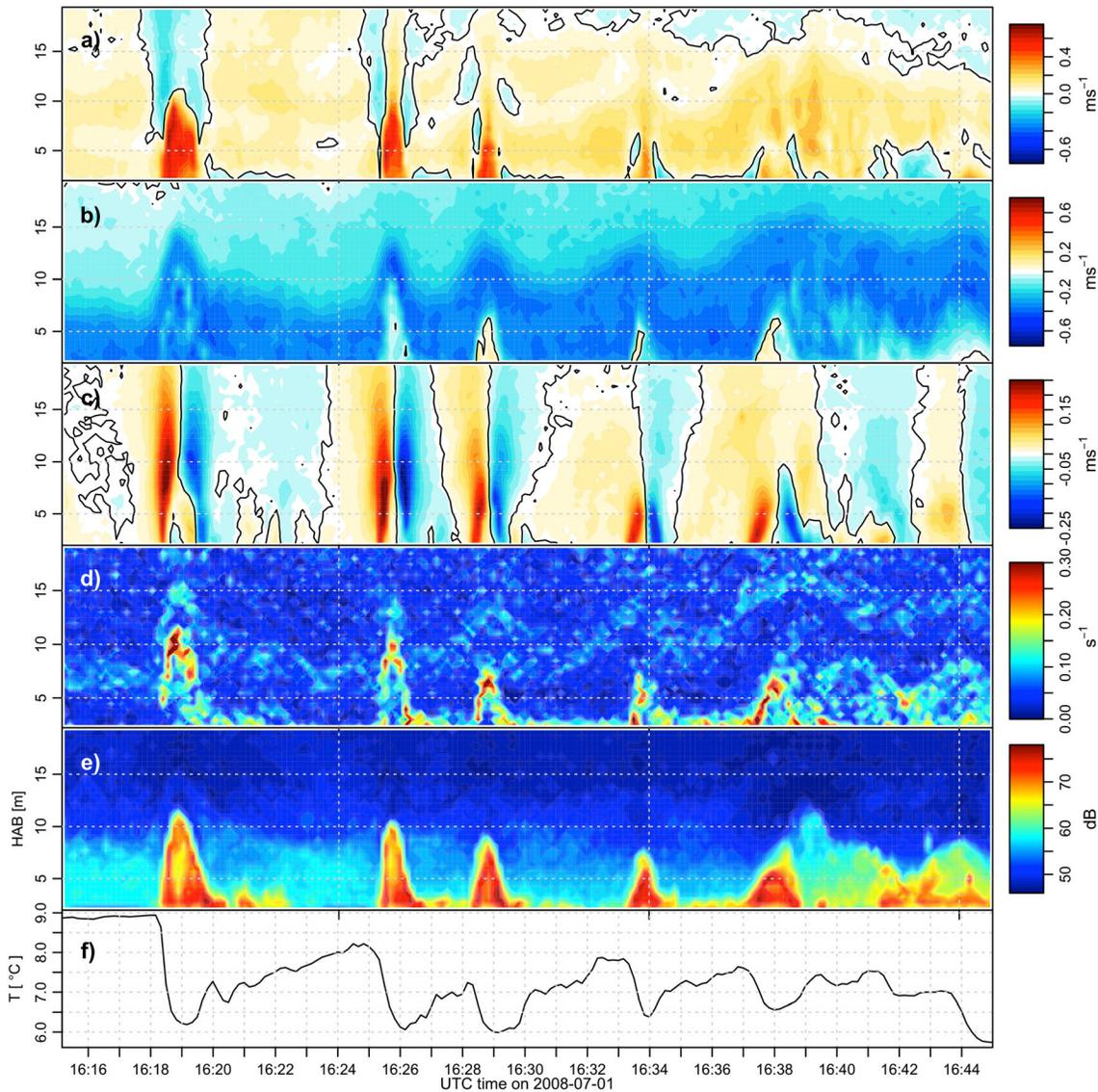
**Figure 9.** A 30 min segment of a wave shoaling event on 1 July as measured by the M07 ADP, showing (a) onshore velocity, (b) alongshore velocity, (c) vertical velocity, (d) magnitude of the vertical shear of the horizontal current, (e) acoustic backscatter, and (f) bottom temperature. The black line in (a), (b), and (c) indicates the zero contour.
