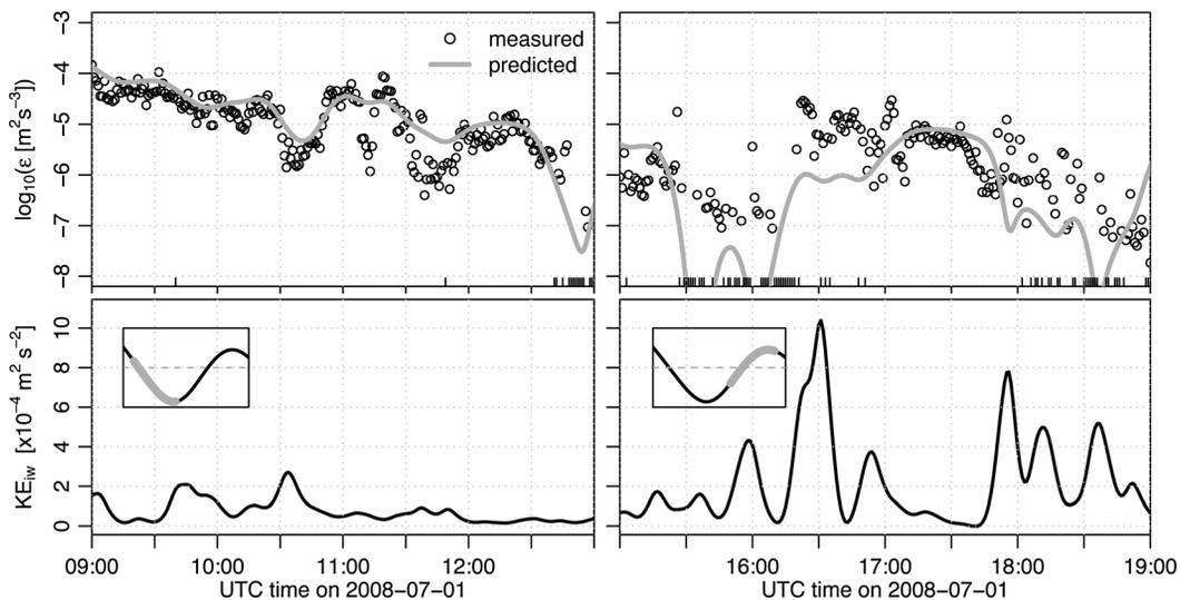
**Figure 11.** Dissipation rates inferred by the Nortek Vector at M05 (circles) and predicted by  $C_D U_f^3 / H$  (gray line) for the two focus periods. Bottom panels show internal-wave activity over the same times, highlighting the periods of low (left) and high (right) internal-wave energy. The phase of the tide is plotted in the inset. The ticks along the bottom of the upper panels indicate times where dissipation values are missing due to the quality control tests.
