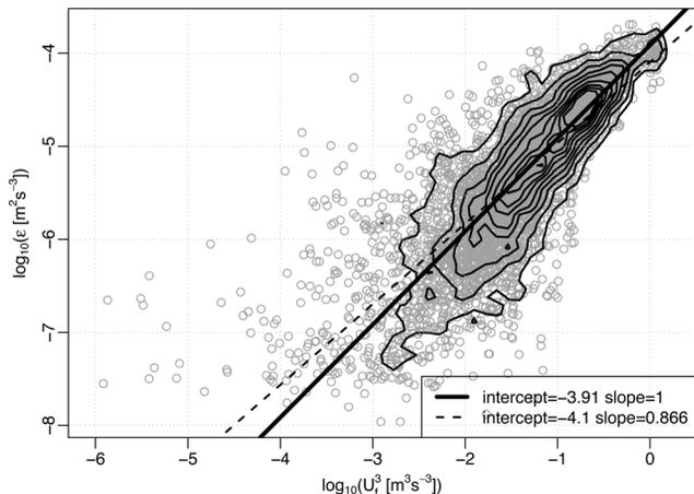
**Figure 6.** Comparison between ADV-derived  $U_f^3$  and  $\epsilon$  for the Nortek Vector at M05. The individual points are plotted as grey circles, while the contours indicate data density (decreasing from 90% to 10%). The solid line is the result of a linear fit with a slope of 1, and the dashed line the result of a linear fit with slope unconstrained. Only points which passed all quality control tests are displayed.
