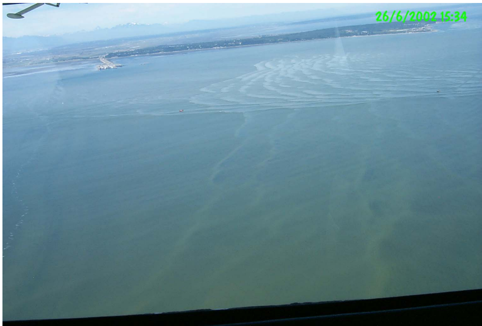
Figure 4. A sample of the original photo images taken on June 26 (interaction Case A). On the image is an oblique top view of two internal wave packets interacting obliquely. A third packet resulting from the interaction is also visible. Slicks are spaced about 200 m apart. The red dot at the center left is the hovercraft.
